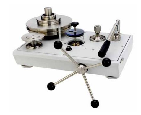
The Pressurements 3000 Series is the culmination of over 50 years experience in the production and design of primary pressure standards. With features designed to improve accuracy and performance, increase reliability and simplify operation these deadweight testers can be used to calibrate virtually any pressure sensing device, including transducers, transmitters, gauges or pressure switches.
