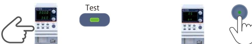
Press the TEST button, read the memory to be executed and press OUTPUT to execute the test script.
