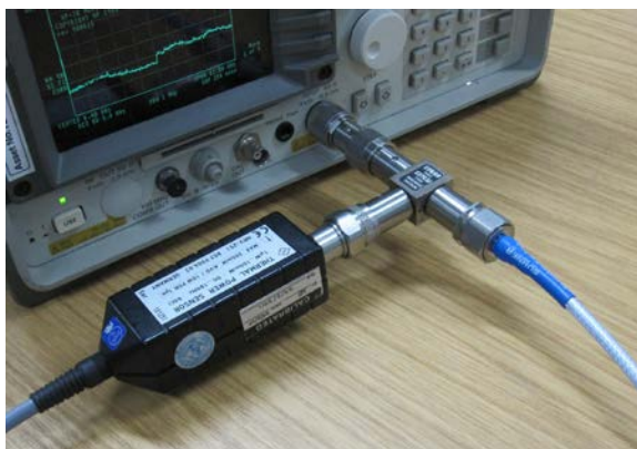
Figure 3. An example of a power splitter employed for precision levelling in a spectrum analyzer calibration application where the device shape and labelling help to easily identify its port configuration.
