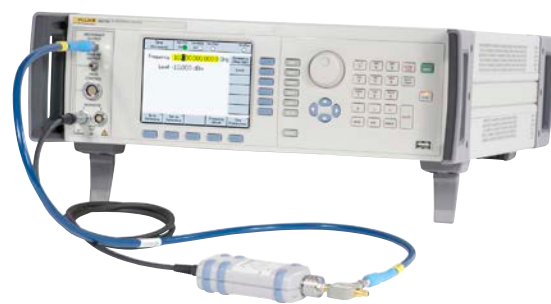
Figure 5. Using an RF reference source like the Fluke Calibration 96270A can help you avoid mistakes and reduce measurement errors. The 96270A delivers an accurate input directly to the UUT up to 27 GHz with its unique "What you set is what you get" feature and ability to "self-characterize" or profile its output to account for losses and attenuation of system components like cables, attenuators, splitters, and connectors, effectively creating a signal reference plane at the UUT input connection.
