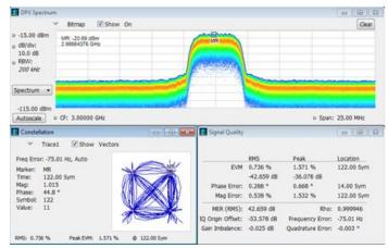
Time-correlated views in multiple domains provide a new level of insight into design problems not possible with conventional analyzers. Here, modulation quality and the constellation measurements are combined with the continuous monitoring of the DPX  $^{\circ}$ spectrum display.
