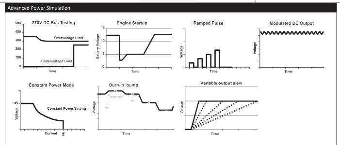
SGX model provides constant power mode allowing independent setting of the max voltage, current and power
