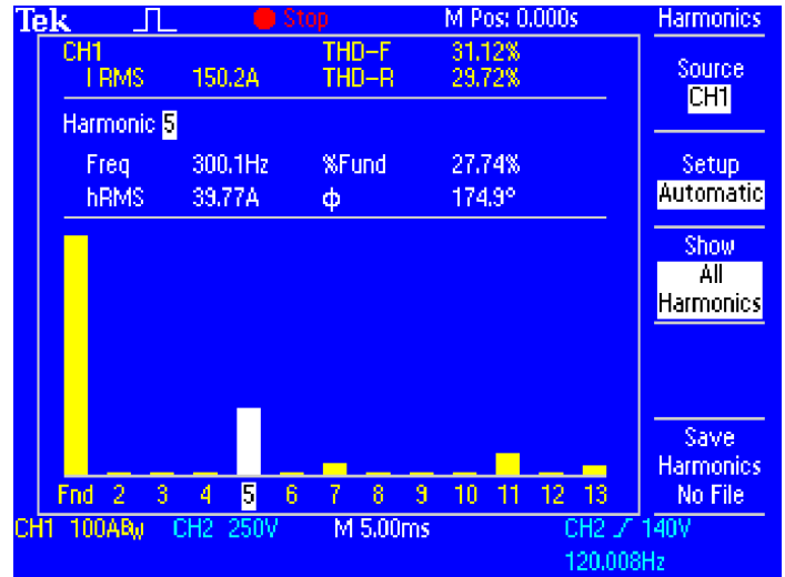
Conduct harmonic distortion measurements with TPS2PWR1 software.
