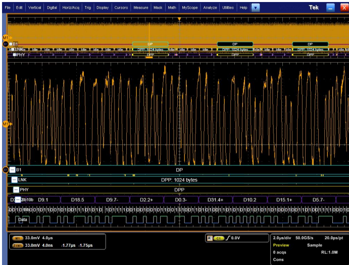
USB 3.0 bus display showing multiple layers simultaneously
