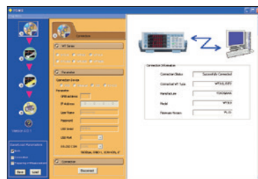
Configuring and Establishing a New Connection between the WT310E and a PC
