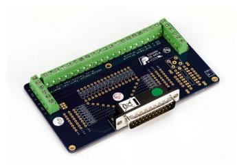
Additionally, the ADC-24 has four configurable digital input/output channels that can be used to control alarms or other devices. The flexibility of the ADC-20 and ADC-24 allows you to use these precision data loggers as an advanced multichannel data acquisition system with a low cost per channel.
