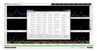
The pulse analysis application license enables you to search for pulses and return all results with start/stop time, average power, peak power, pulse duration, PRI and start/stop frequencies. Pulse parameters can be exported as PDWs or emrk for use with other tools.
