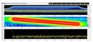
In the illustration above, analysis is performed with the base application license for DataVu-PC. The signal is a linear frequency chirp of 10 usec duration, 700 MHz bandwidth acquired with the RSA7100A. The spectrogram analysis is set to 99% FFT overlap on a pulse of 10 usec duration.
