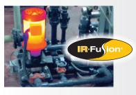
The 3.5" LCD touchscreen offers IR-Fusion™ to blend a visible light image with an infrared image to more easily locate problems. Simply slide your finger across the screen to adjust the setting.
