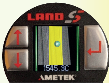
Temperature measurement data from the SPOT pyrometer
