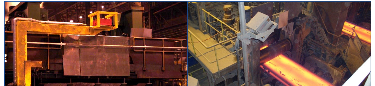
The LSP-HD linescanner in the hot rolling mill
