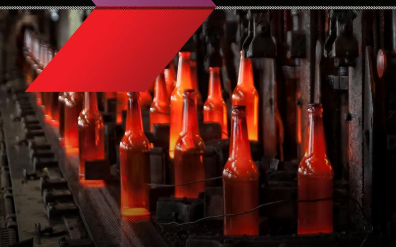
Accurate and reliable temperature measurements at key process locations are vital to ensure consistent quality throughout container glass manufacture.
